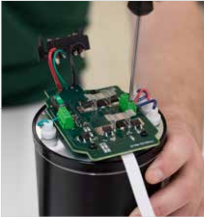
Loosen the four screws that hold the feedthrough wires in place.
