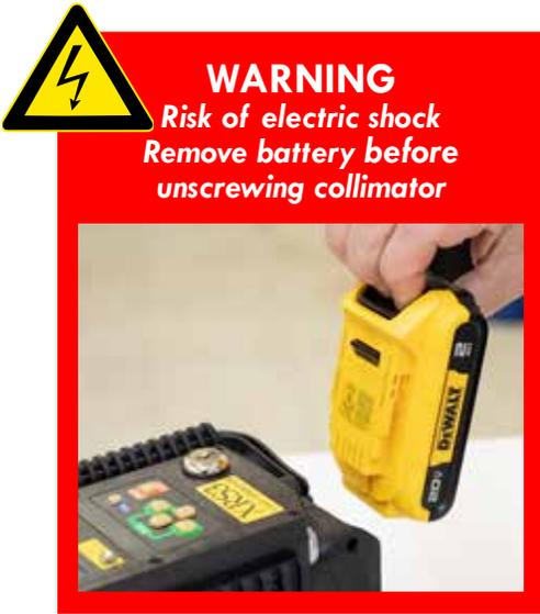
1. Remove the battery before unscrewing the collimator.
