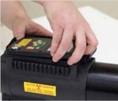
Lift the top plate from the front (nose) of the unit.
