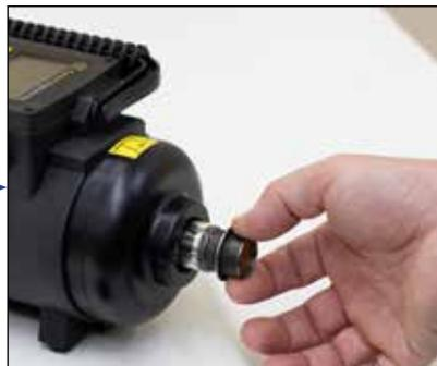
Grip the front of the tube and pull straight out
