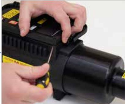
Gently pry the front of the control module with a flat screwdriver.
