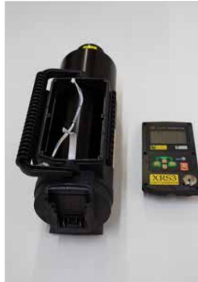
The Control Module is removed.
