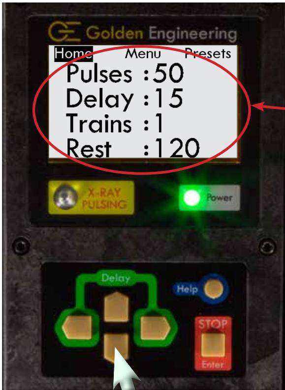
This is the HOME screen. From here you can set the number of pulses, delay in seconds, and adjust the trains settings. See MANUALLY ENTERING PULSE TRAINS.
