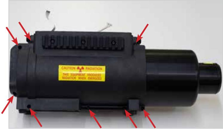
Remove the screws that hold the housing together
