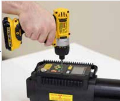
Use T10 Torx driver to remove 6 screws holding control module in place.
