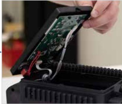
Tip the plate toward the battery to expose the wires.
