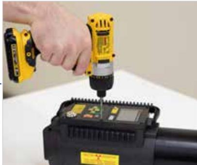
Use T10 Torx driver to remove 6 screws holding control module in place.
