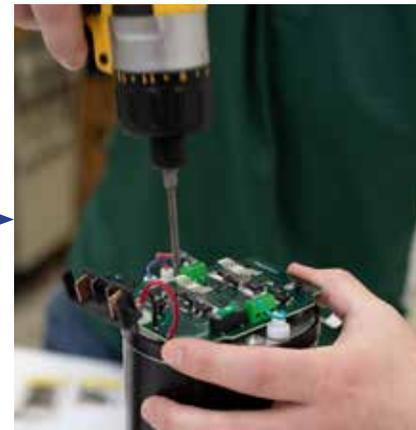
Remove the oscillator board.
