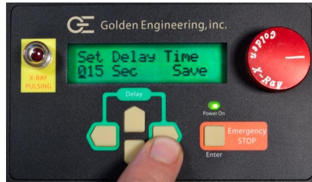
Use Left/Right arrows to select digit Use UP/DOWN arrows to change number Delay option from 5 to 240 seconds
