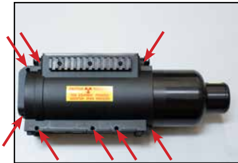
Remove the screws that hold the housing together XR200 and XRS3 both have 8 screws; XRS4 has 7 in the main body, plus another 8 in the handle
