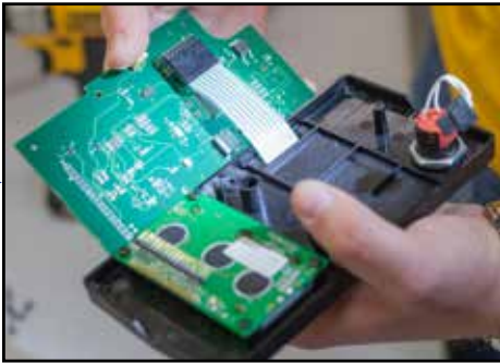
Disconnect ribbon cable.
