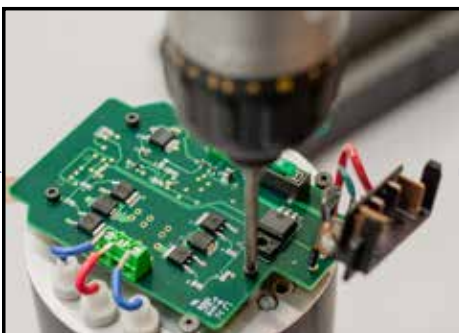
Remove the screws that connect the oscillator board to the head.
