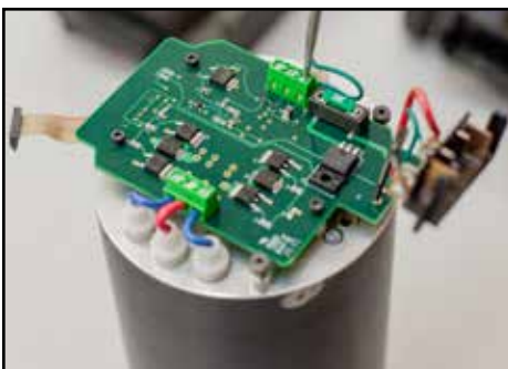
Loosen the four screws that hold the feedback wires in place.
