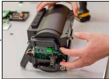
Remove one side of the housing.
