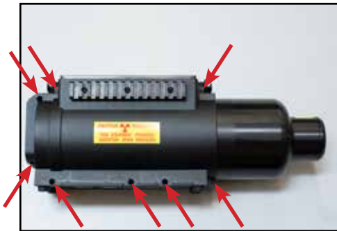
Remove the screws that hold the housing together. XRS3RA has 8 screws; XRS4RA has 7 in the main body, plus another 8 in the handle
