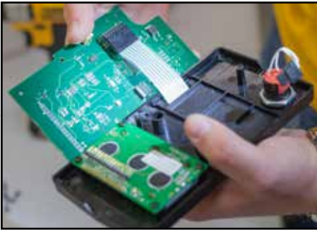
Disconnect ribbon cable.
