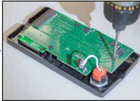
Remove 3 screws holding processor board to top
